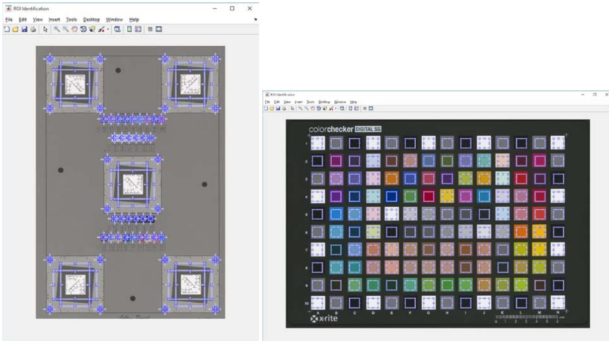
Figure 2. Target regions of interest for imaging quality factor measurements
